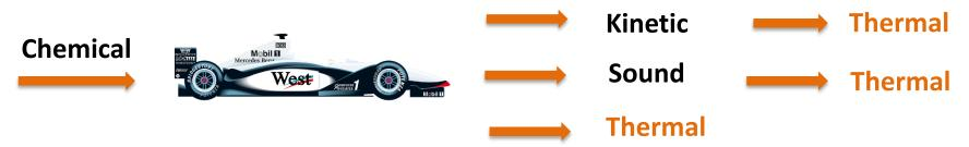
Kinetic energy is dissipated by the tyres, brakes and air resistance to become <u>unwanted</u> thermal energy stores.
