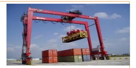
The crane lifts the 2000 kg container through a height of 5.4m in 30s. The power of the crane is: Power = Work / time But: Work = force x distance
