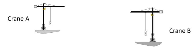
Crane A takes 30 s to lift the load. Crane B lifts the same load in 9 s.
