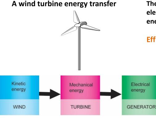
The wind turbine produces 120 MW of electrical energy for every 500 MW of kinetic energy provided by the wind.
